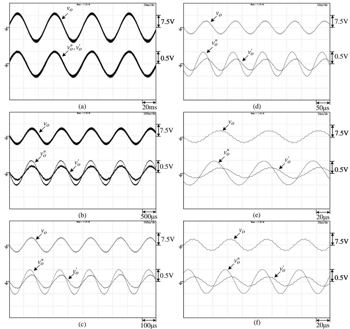
Fig. 5.1. Measured  $v_o$  and  $(v_o^*, v_o')$  of the established full-bridge inverter under  $R_o = 10\Omega$  and  $v_{cont} = 0.5\sin(2\pi f_1 t)$  without voltage robust controller: (a)  $f_1 = 20\text{Hz}$ ; (b)  $f_1 = 1\text{kHz}$ ; (c)  $f_1 = 5\text{kHz}$ ; (d)  $f_1 = 10\text{kHz}$ ; (e)  $f_1 = 15\text{kHz}$ ; (f)  $f_1 = 20\text{kHz}$
