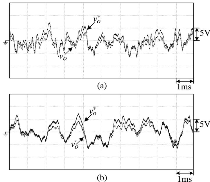
Fig. 5.4. Measured ( $v_o^*, v_o'$ ) of the established H-bridge inverter with audio signal from CD player using loudspeaker: (a) without VRECC; (b) with VRECC.
