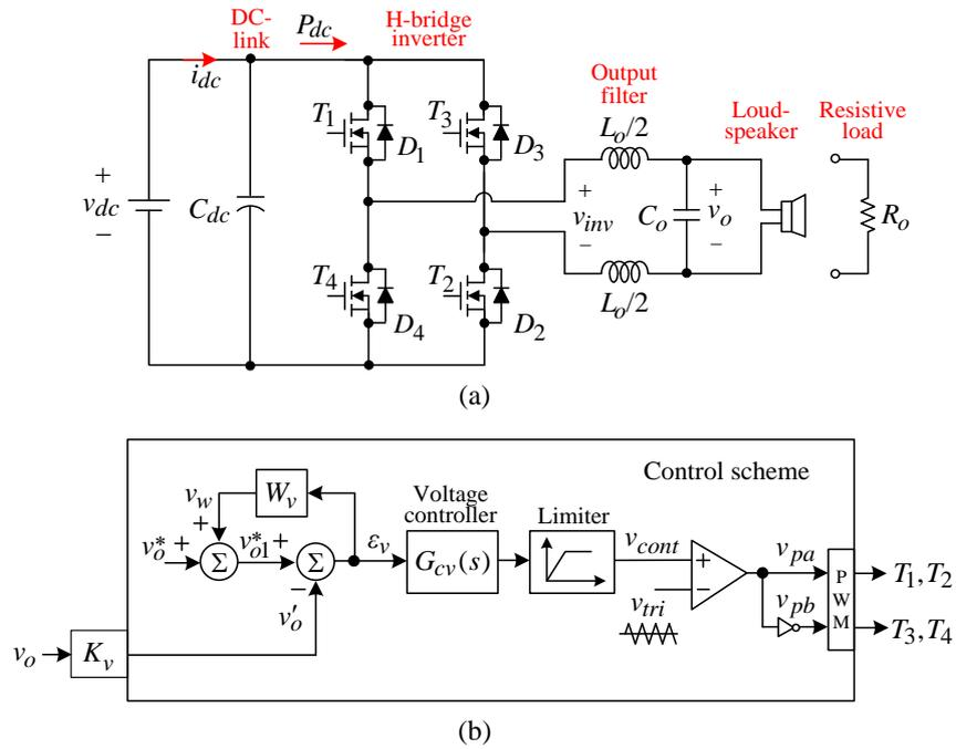
Fig. 1. The established Class-D audio amplifier: (a) power circuit; (b) control scheme.
