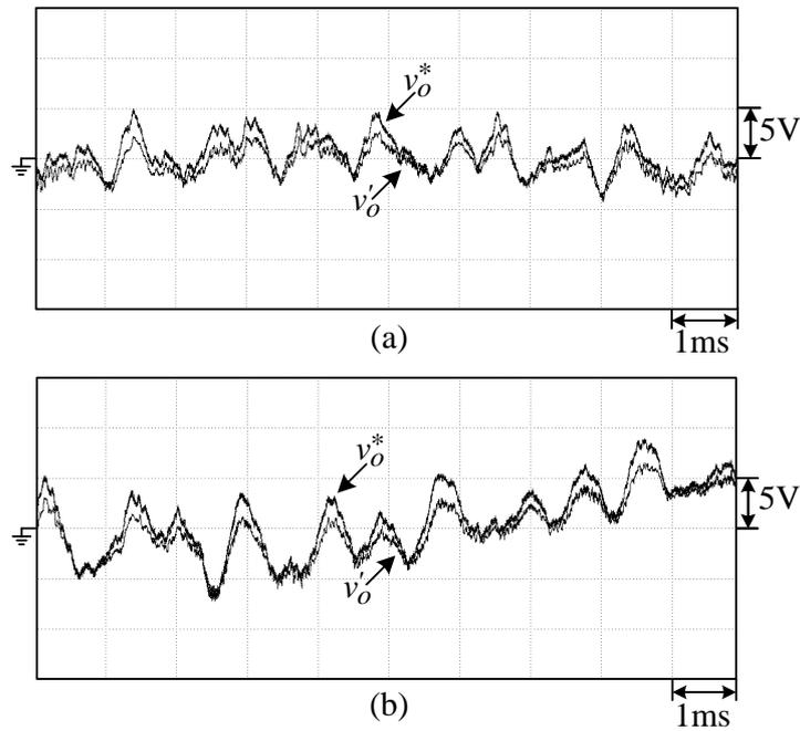
Fig. 5.3. Measured ( $v_o^*, v_o'$ ) of the established H-bridge inverter with audio signal from CD player: (a) without VRECC; (b) with VRECC.
