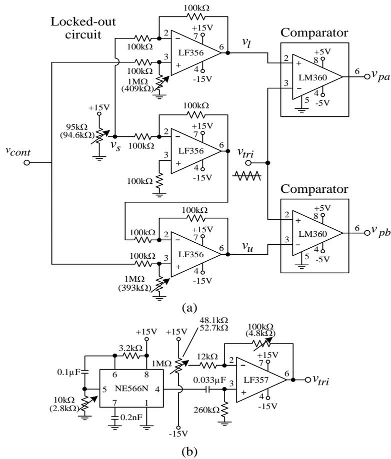
Fig. 2. Analog implementation circuit of open-loop control scheme: (a) dead-time setting; (b) triangular carrier wave generator.
