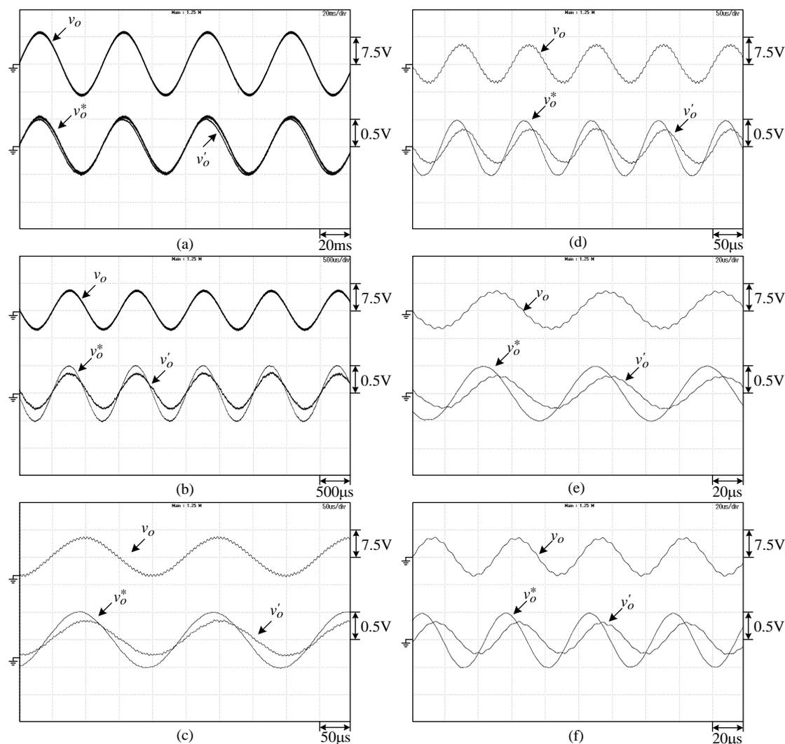
Fig. 5.2. Measured  $v_o$  and  $(v_o^*, v_o')$  of the established H-bridge inverter under  $R_o = 10\Omega$  and  $v_{cont} = 0.5\sin(2\pi f_1 t)$  with voltage robust controller: (a)  $f_1 = 20\text{Hz}$ ; (b)  $f_1 = 1\text{kHz}$ ; (c)  $f_1 = 5\text{kHz}$ ; (d)  $f_1 = 10\text{kHz}$ ; (e)  $f_1 = 15\text{kHz}$ ; (f)  $f_1 = 20\text{kHz}$ .
