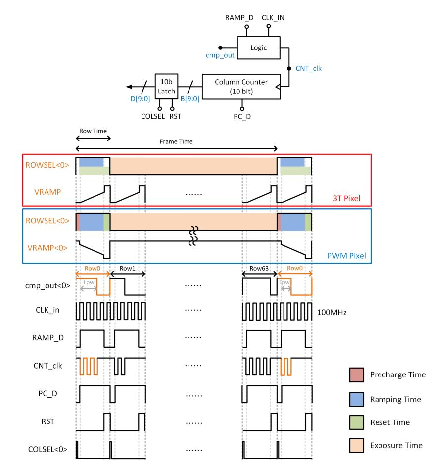
This study adopts a rolling shutter readout method, where rowsel<n> sequentially selects each row for readout. The diagram on the left illustrates this process using row0 as an example.
