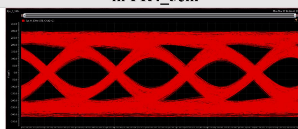
PAM4 eye diagram before compensation in FR4_5cm
