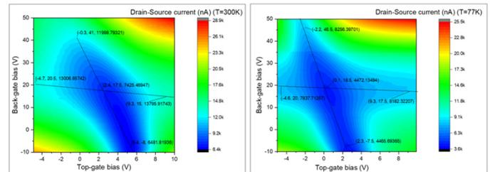
Fig. 3 Measurement of the two-dimensional current map for the device with back gate-upper gate bias.
