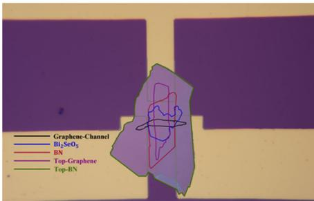
Fig. 1 The schematic design drawn from existing samples.
