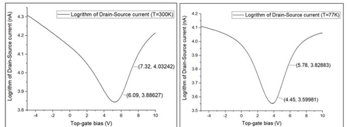
Fig. 4 Subthreshold swing determination
