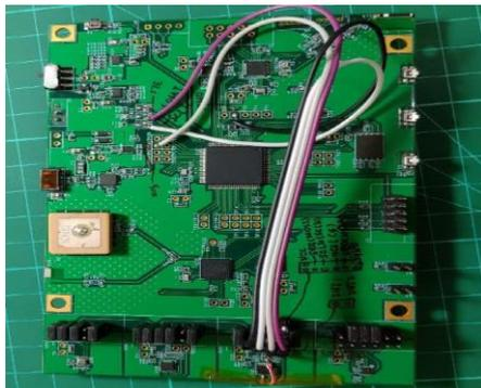
Figure1. PCB for SPI control
