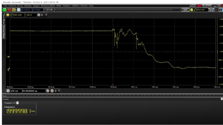
Fig. 8 Fall Time of the MC74AC14 Hex Inverter Schmitt Trigger
