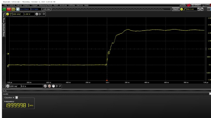
Fig. 9 Rise Time of the MC74AC14 Hex Inverter Schmitt Trigger
