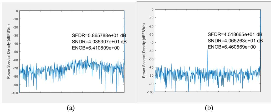
**Fig. 4. The spectrum with purposely added timing mismatch (a) RIS on(b) RIS off**
