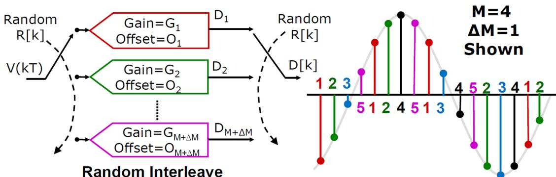
**Fig. 1. The Random Interleaved Sampling (RIS) Method to smear the spurious components by randomness, when channel mismatch exists**
