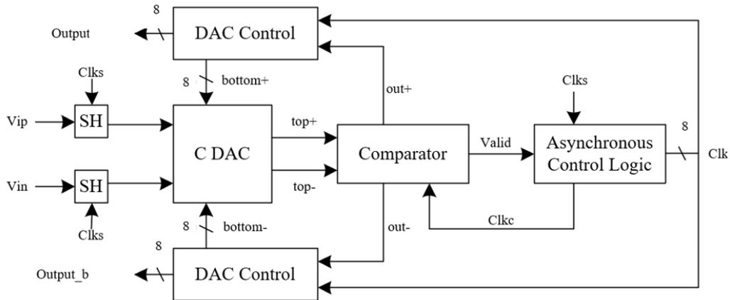
**Fig. 3. The block diagram of single channel SAR ADC**
