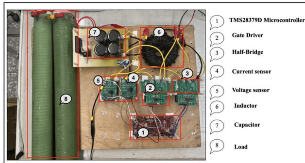
Figure 8: Physical circuit
