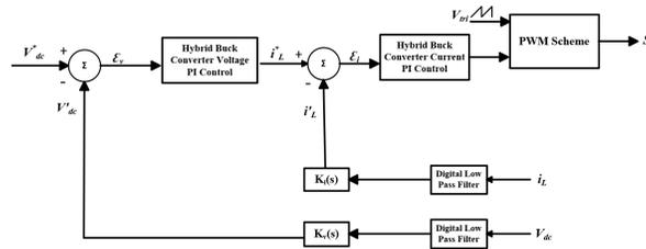
Figure 12: Hybrid Buck Converter Closed Loop Control
