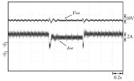
Figure 15: Step load change  $10\Omega \rightarrow 15\Omega \rightarrow 10\Omega$
