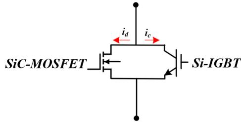
Figure 3: SiC-MOSFET/Si-IGBT Hybrid Switch
