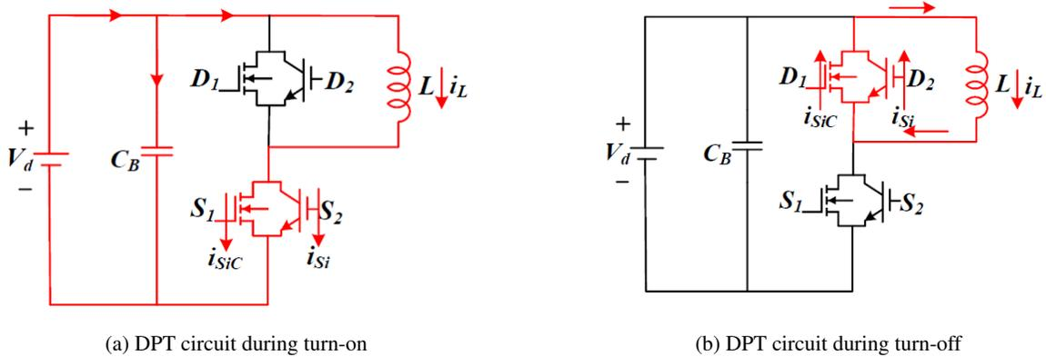
Figure 2: DPT Switching Characteristics: (a) ON and (b) OFF
