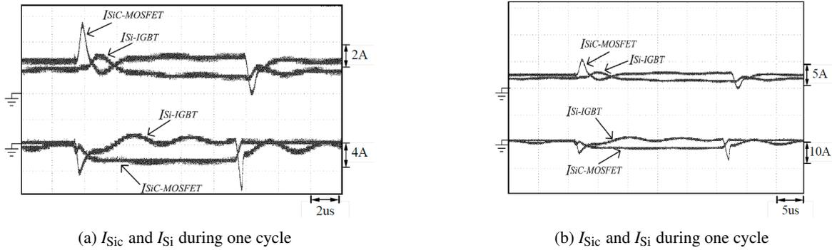
Figure 11: Switching Characteristics: (a) Current sharing 2A/4A scale and (b) Current sharing 5A/10A scale
