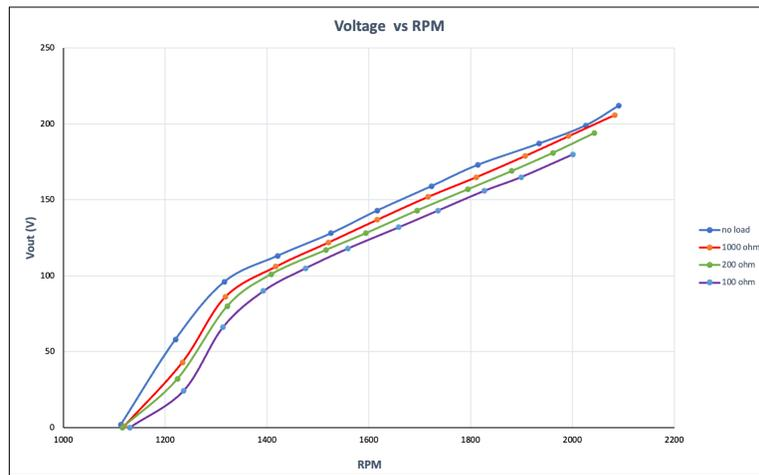
Figure 18: Motor speed and Output Voltage of generator with different load.
