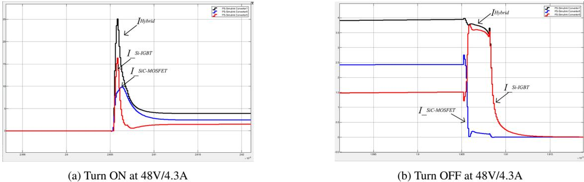
Figure 4: Switching Characteristics: (a) Turn-on and (b) Turn-off waveforms
