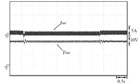
Figure 16: Step load change  $10\Omega \rightarrow 15\Omega \rightarrow 10\Omega$
