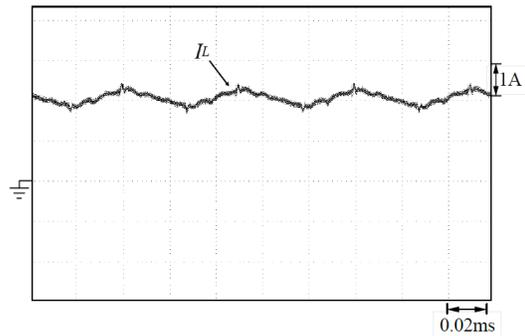
Figure 14: Inductor current  $I_L$
