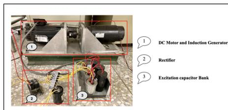
Figure 17: Wind generation setup
