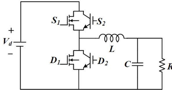
Figure 7: Hybrid Buck Converter Topology
