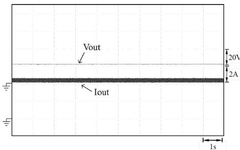
Figure 9:  $V_{out}$  24V and  $I_{out}$  4.3A Steady State
